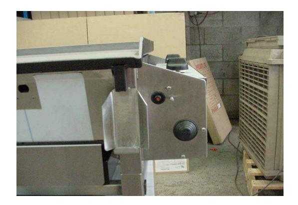
Barbecue showing the Heatlie Timer. This can only be added to a Flame Failure BBQ at the time of Manufacture. Additional time will be needed to manufacture this BBQ.
